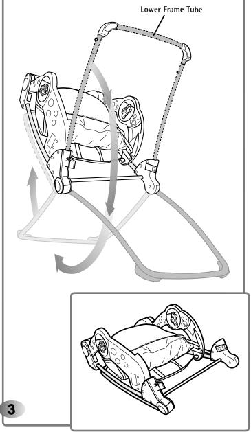
• Rotate the lower frame tube around to the top of frame, as shown.
